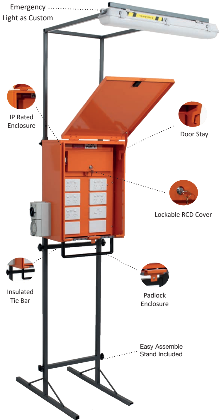
*Image: TPB-3PT5.532 with Custom LED IP65 Emergency Light
